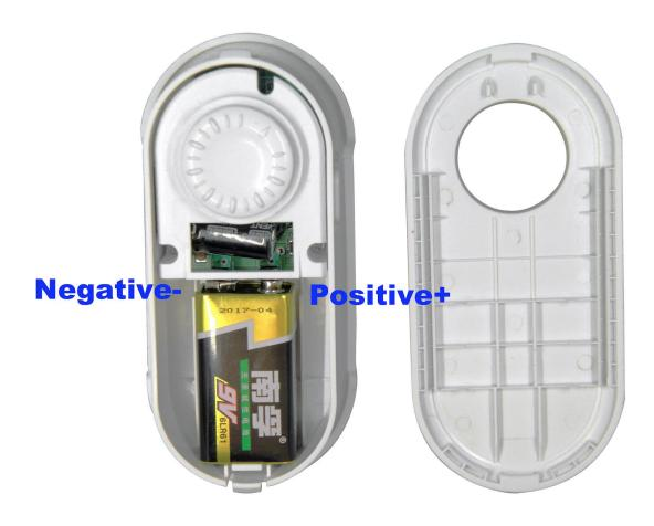
Position the lid so the top is held by a tab on the main unit, and gently click the lid shut. Do not use excessive force.
